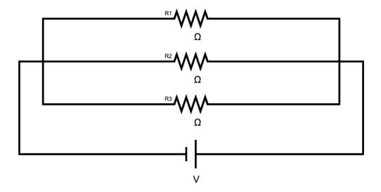
Step 2: Calculate the current for each of the resistors. Show your work for one of these in the space below and then draw the currents into your picture above.
