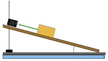
Step 2: Calculate the force gravity on the block and then figure out the Fgx and the Fgy when you rotate your axes to match the angle of the incline. Then calculate the Fn, the Ff, and the Ft. Put all these forces into the picture shown below. Show all your work for these calculations. Check your work by trying your answers in the program.
