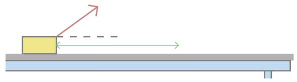
Step 2: Draw in all the forces on your object. Then calculate the force gravity, resolve force tension into components, calculate force normal, and finally calculate the force of friction
