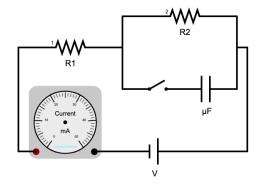
Step 2: Fill in the voltage of the battery and the capacitance of the capacitor. Then use arrows to show the flow of electricity through the circuit while the switch is first closed and the capacitor is still uncharged as shown below. Also show the location of the needle when the switch is first closed. Calculate the value of R1 and then determine R2
