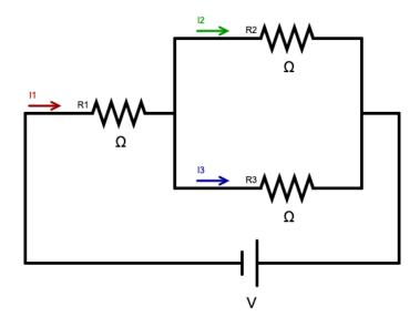
Step 2: Calculate the total resistance and the total current in the circuit. Show your work neatly below.
