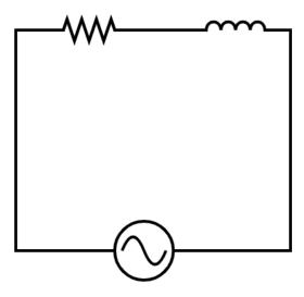
Step 2: Calculate the effective impedance of the circuit. Show your work below.
